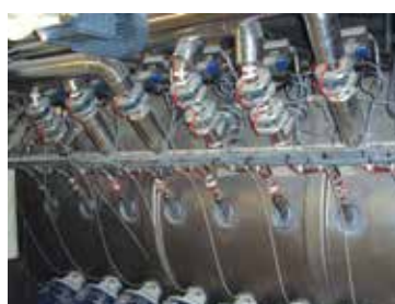
Choppers, liquid injectors, temperature jacket
